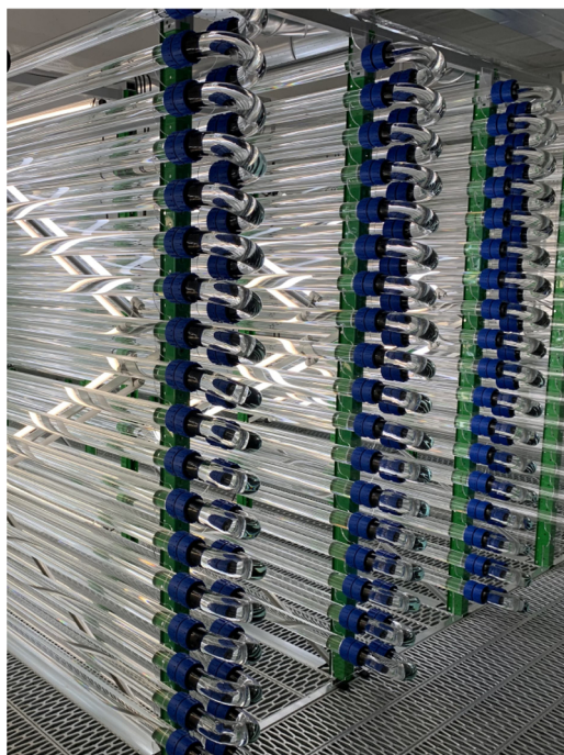
Fig. 2. Tubular photobioreactor arrangement. Source: the authors.
